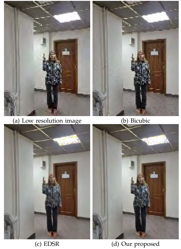
Figure 1. Comparison of gesture recognition results on a \times 4 super-resolved image using different methods. The YOLOv10 detector assigns varying confidence scores depending on the input quality. Our proposed method achieves the highest confidence (0.86), outperforming Bicubic (0.74), EDSR (0.69), and the original low-resolution input.
